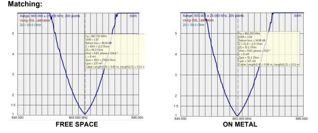
The graphs above show the typical EU VSWR, the US VSWR is approximately the same. The closer the curve is to the bottom line the closer the antenna is to a 50 Ohm input match. If the antenna was perfectly matched to 50 Ohms then all the energy would radiate from the antenna and none would be reflected back to the reader. The design inherently maintains VSWR when re-tuned to other frequencies. (A 'VSWR' better than 2 is acceptable in most RFID systems.)
